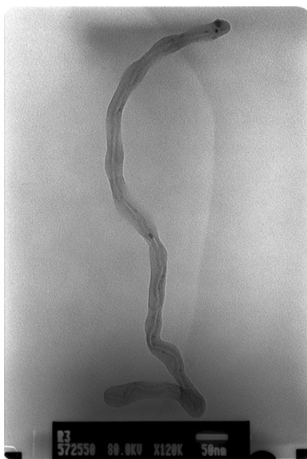
FIGURE 1 Visualization of a typical MWNT by means of TEM which was used for measurements.
